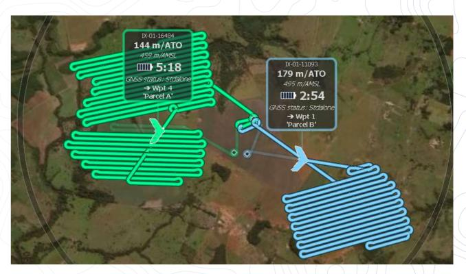
With eMotion, flights are built using mission blocks. Just choose your block, highlight the region you want to map, define key settings, and eMotion auto-generates your drone's flight plan. Multi-flight missions are supported and you can activate/import elevation data for even safer, terrain-accurate flights.
